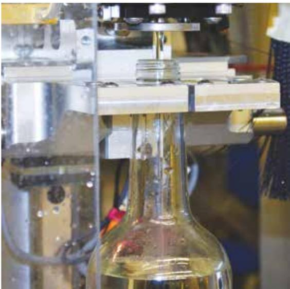
Agr SPT2 incorporates an integrated volume measurement system that performs volume measurements simultaneously with pressure testing, on the plant floor, with laboratory accuracy.
