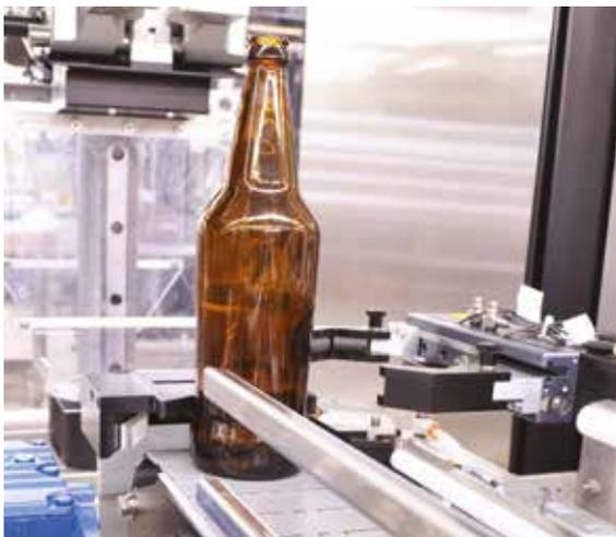
A robotic handling system and universal bottle holders accommodate a range of bottle sizes, without job changes.
