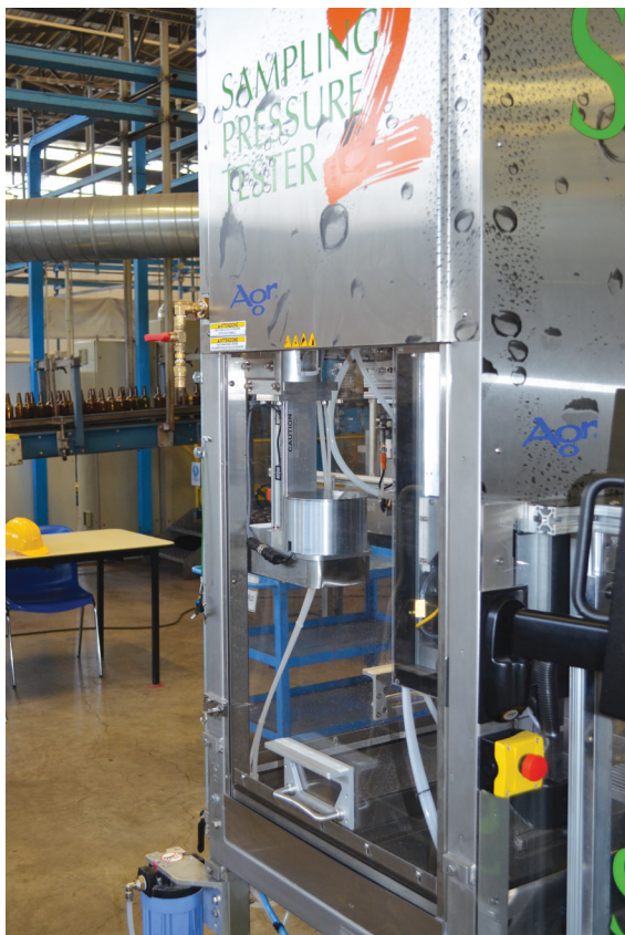
Agr's SPT2 automated volume measurement and pressure testing system, introduced at Verallia Italy's Villa Poma plant.
